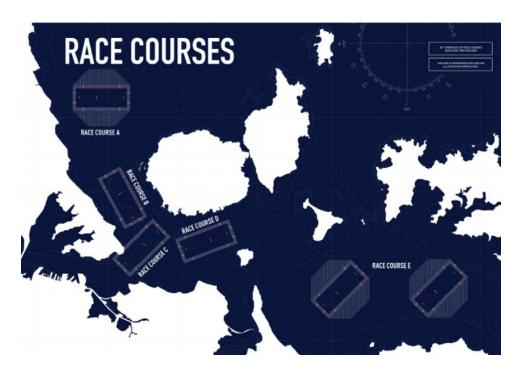
Five race courses were designed by ACE for AC36 in the Waitematā Harbour and Hauraki Gulf (see Figure 4). Each course had a windward-leeward configuration and an upwind start. The length of each course was dependent on location and the prevailing weather conditions, but ranged between 1.1 to 2.2 nautical miles. The course on which the teams sailed was decided on each race day by the Race Director and Race Management, in consultation with the Harbourmaster.
